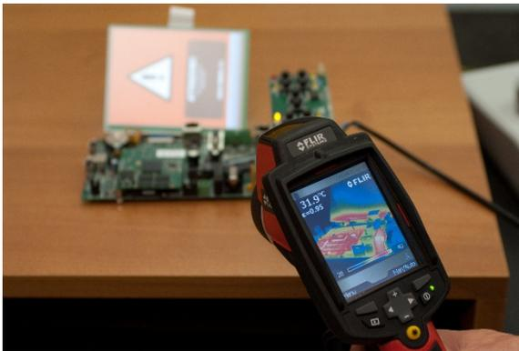
The operating temperature of the board's various components influences their average lifetime. Excessively high temperatures can significantly reduce the lifespan of the components and compromise their general reliability.
